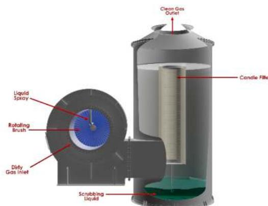
**Figure 4.** Becoflex BFCF schematic.
