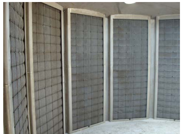
Inside View of Vertical Demister Panel Polygon
