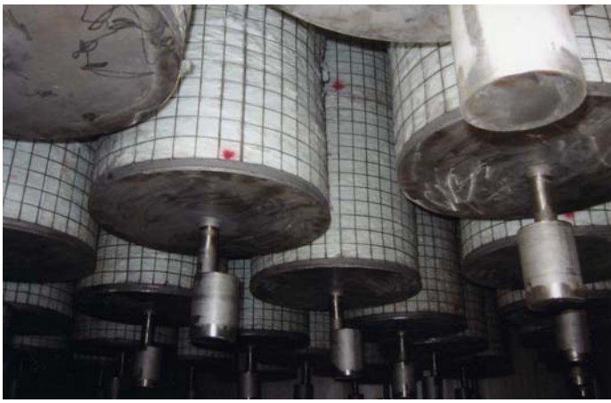
View of hanging type candle filters from below
