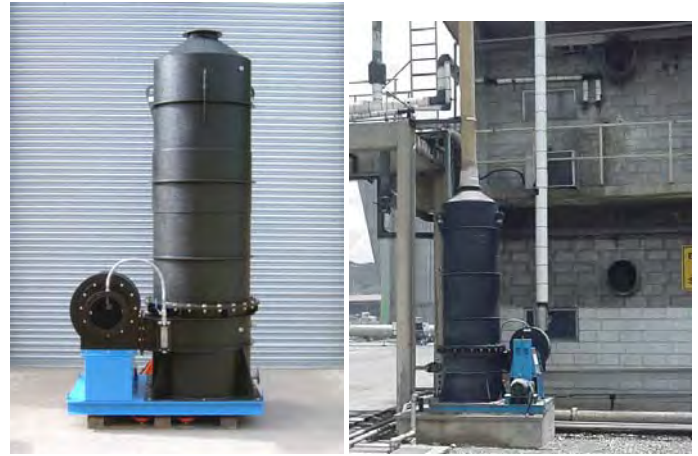
Becoflex BFCF unit on Oleum tanker loading duty
