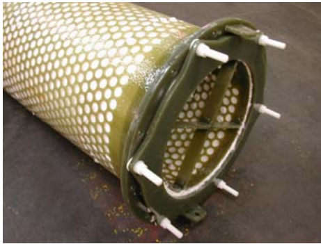
Candle Filter in a GRP + Derakane Resin Structure
