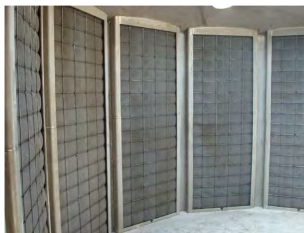
Inside View of Vertical Demister Panel Polygon
