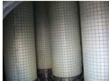
B14W Glass Rope Standing Candle Filters
