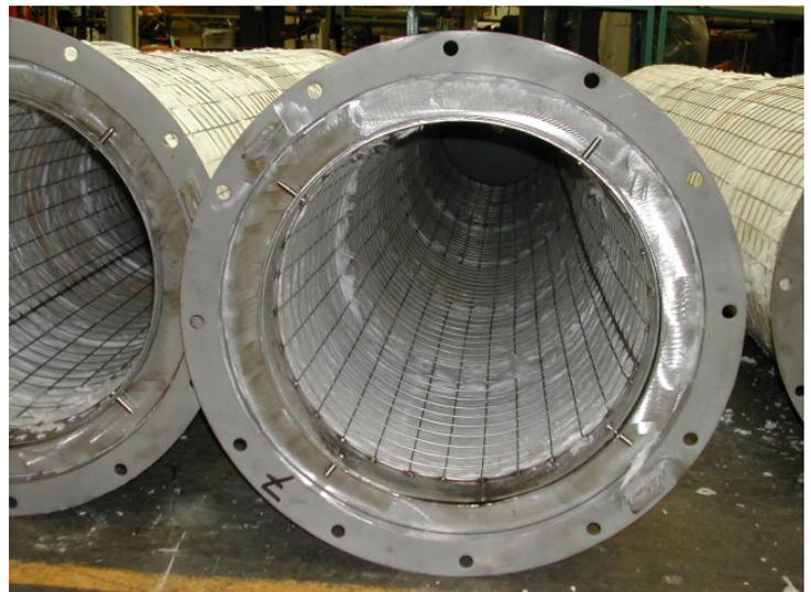
Begg Cousland has always used a technology of preformed elements packed into a 5 centimetre annular space between two concentric cylinders fabricated from corrosion resistant mesh. The candles are installed vertically and gases pass horizontally through the filter wall, the trapped particles coalescing and draining down through the filter bed.
