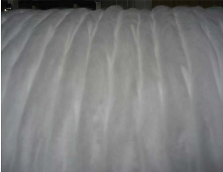
These B14W mist eliminators can be made in 3 depths – 50, 63 or 75mm – and can be supplied with or without an exit surface drainage mat layer. This means we can adapt our beds to meet the demands of different high mist load duties. We can also repack the structures of other suppliers.
