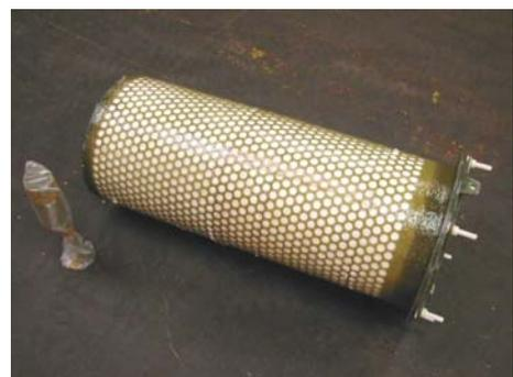
Wet Chlorine Gas filter with GRP structure
