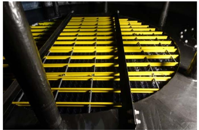
A Vertical Scrubber with BlueFil® Mesh Packing.
