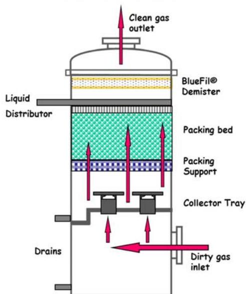
Some Fluorine scrubbers are vertical and, like the above image of a Granulator Tail Gas Scrubber, can have a 1<sup>st</sup> stage random packing bed with liquid distributor counter-current followed by a horizontal BlueFil® Meshpad.
